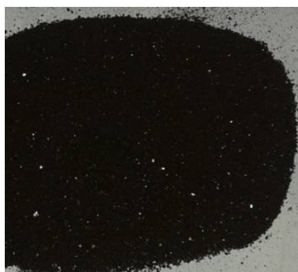
Fig.3. Biosynthesized Copper Nanoparticles from Arecanut Extract
